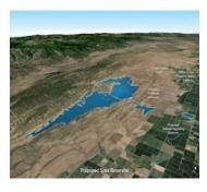
Sites is a proposed off-stream reservoir located northwest of Sacramento that would provide 470,000 to 640,000 acre-feet of water storage and improve water supply reliability and flexibility in the system.
