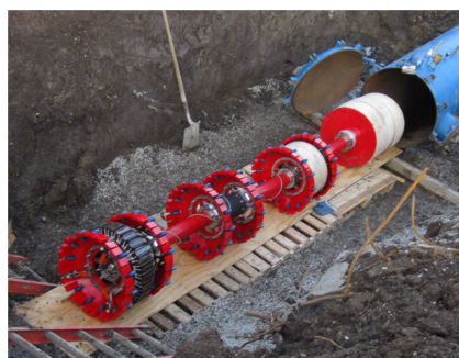
Internal Condition Assessment Advanced NDT Remote Field Testing (RFT)
